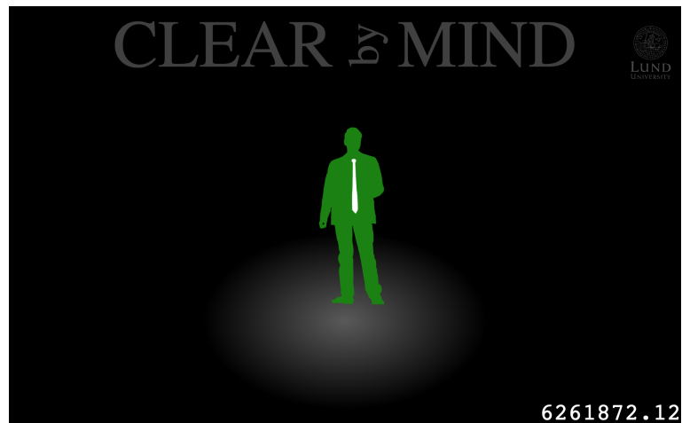
Figure 5. Screenshot of client GUI, where the subject is asked to focus on the visual stimuli which changes a number of times per second during a session. In this case, in the BCI-HIL Clear By Mind example application (see Section 4.2 for details).
